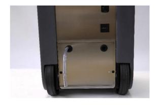
⇒ If necessary, extend the hose to the intended collection container or drain.
